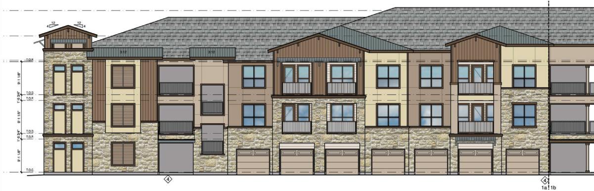
1a BUILDING TYPE 'C' - ELEVATION SCALE: 1/8" = 1'-0"
