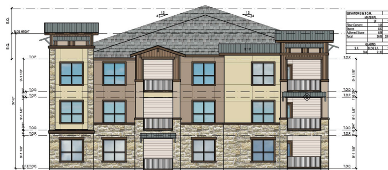
3 BUILDING TYPE 'C' - TWO ELEVATIONS (ONE O.H.) SCALE: 1/8" = 1'-0"
