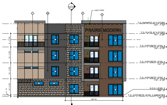
1 EXTERIOR NORTH ELEVATION - 1 1/8" = 1'-0"
