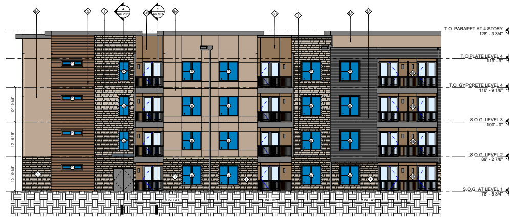
2 EXTERIOR SOUTH ELEVATION - 2 1/8" = 1'-0"
