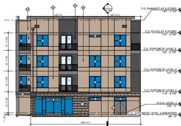
2 EXTERIOR EAST ELEVATION - 1 1/8" = 1'-0"
