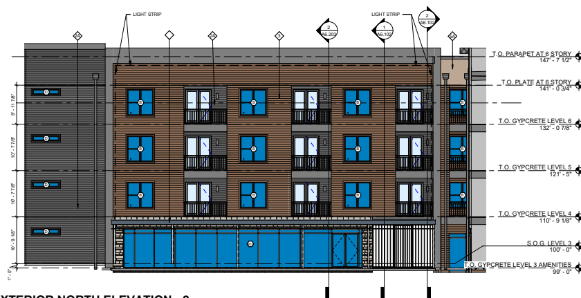
3 EXTERIOR NORTH ELEVATION - 2 1/8" = 1'-0"
