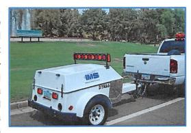
rating. These readings will then be used to determine the pavement strength, load transfer capabilities, and identify properties of the base and sub-grade.
