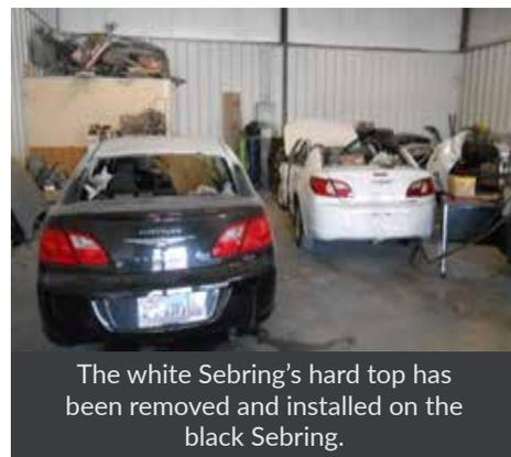
The white Sebring's hard top has been removed and installed on the black Sebring.
