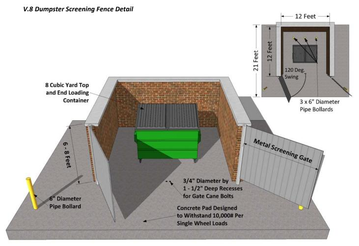
Note: The cast stone cap show in the diagram above is optional. The above detail shows a concrete pad underneath the screening wall. This pad is only necessary when an approved concrete surface area is not present on the site.
