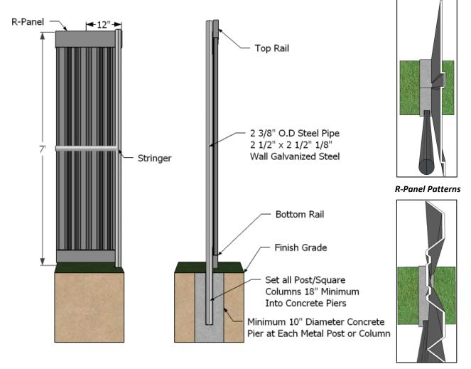
**Note:** Detail shows the front, top and side elevations of an R-Panel section for a recommended metal fence to be constructed in the Light Industrial-Limited Standards (LI-LS) District. Appropriate screening designs for this district may include several variations of R-Panel provided that in any case the metal screening is visually non-transparent. Corrugated metal is not an approved fencing material.
