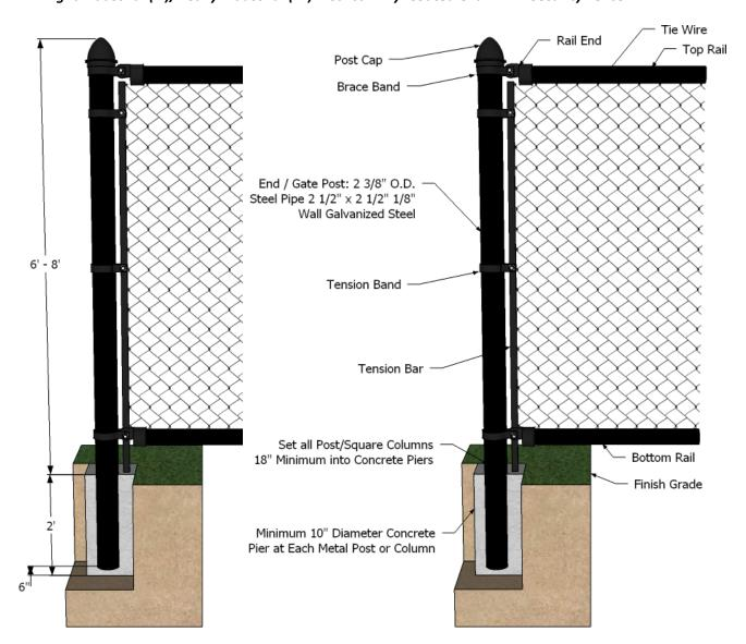
**Note:** Detail shows the side elevation of a Vinyl Coated Chain Link Security Fence section and the elements necessary for the fence to be constructed on the property line in the Light Industrial (LI) District. Uncoated steel or galvanized fencing will not be permitted to be situated on the property line.
