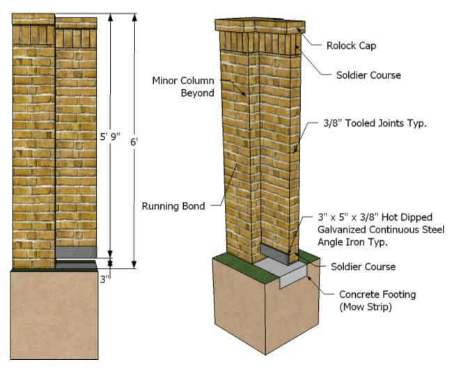
**Note:** Detail shows the front and side elevations of a column and wall section for a masonry-screening wall. Appropriate masonry screen designs may include pre-cast panels or panel sections, or other, provided that in any case the masonry screen is visually non-transparent.
