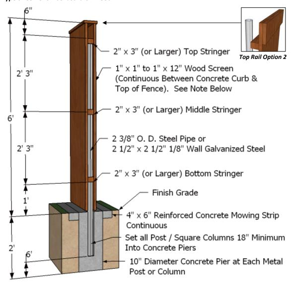
**Note:** Detail shows finish surfacing on both sides, surfacing on one side is acceptable. Appropriate wood screen designs may include board on board, board & batten, solid panel, or other, provided that in any case the wood screen is visually non-transparent.
