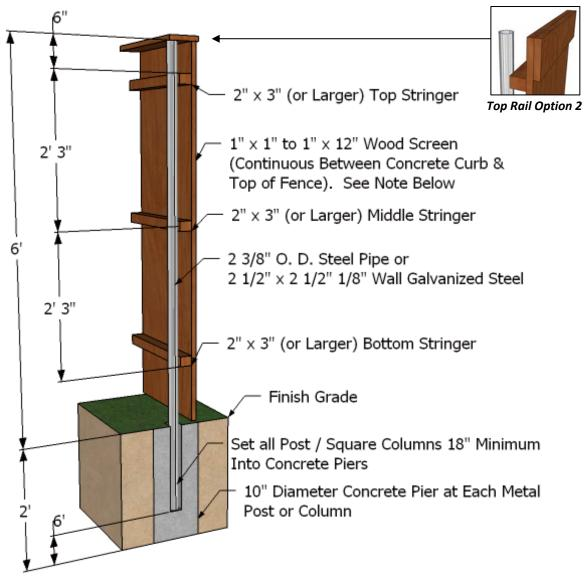
**Note:** Detail shows finish surfacing on both sides, surfacing on one side is acceptable. Appropriate wood screen designs may include board on board, board & batten, solid panel, or other, provided that in any case the wood screen is visually non-transparent.
