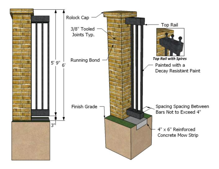
**Note:** Detail shows the front and side elevations of a masonry column and wrought iron section for a Type 2 screening fence. Where a masonry column is not required a wrought iron column may be used. Spires or other appropriate decorative fencing elements may be used as long as they do not cause the fence to exceed the maximum/minimum height restrictions.
